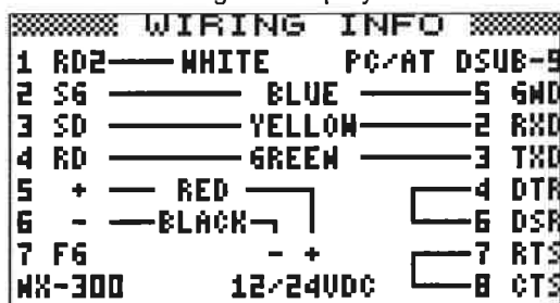
Figure 2-15 Connection to PC using a DSUB 9-pin connector
