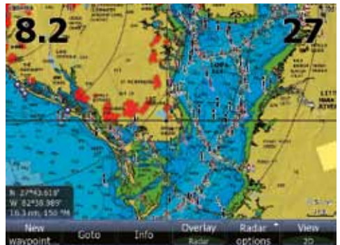
Broadband 4G Radar detects many separated cells inside a Florida rain storm overlaid on a chart greater than 16nm away
