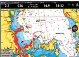
Broadband 4G Radar clearly detects the New Zealand Coromandel Peninsula .>29nm away with the B&G Zeus
