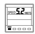
Press **SPEED** key to display current boat speed.
