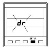
Press **SETUP** key 6 times to display **dr**. The display will flash.
