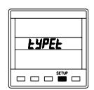
Press **SETUP** key to display the current mode.
