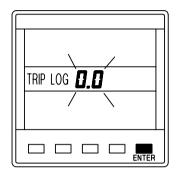
Press **ENTER** key, the display resets to zero, and remains flashing.
