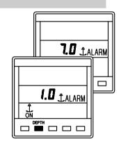
Press DEPTH key to display the anchor alarm.
