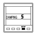
Press **SETUP** key once to display the damping value.
