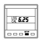
Press **SETUP** key four times to display **LOG CAL**
