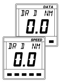
The **dr** log will be reset to zero when displayed on SPEED or DATA units.
