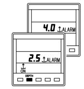
Press **DEPTH** key to display **ANCHOR ALARM**
