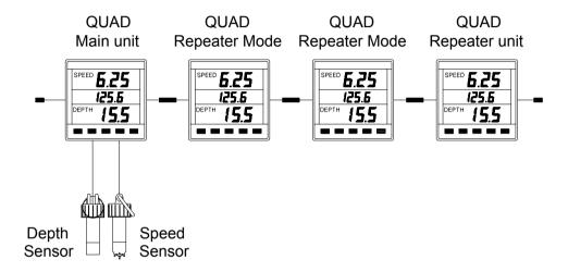
When in repeater mode, if the data is not being received from the system network, the display will show OFF when a key is pressed.
