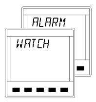
The Off Course alarm is activated when the boat deviates off course by a preset amount. The display alternates between the messages below:
