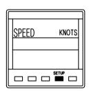
Press **SETUP** key twice. The speed digits will blank.
