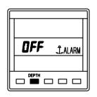
Press **DEPTH** key to display anchor alarm.
