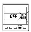
Press **SETUP** key, the alarm state will be displayed.
