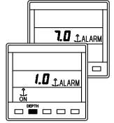
Press DEPTH key to display the anchor alarm.
