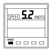
Press **SPEED** key to display the current boat speed.
