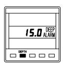
Press **DEPTH** key, the value is displayed and the alarm enabled.
